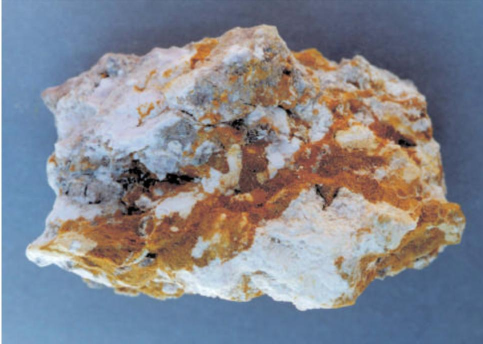
**Figure 10. Hand sample, 7 x 9 cm, showing golden metavoltine vein in fine-grained coquimbite.**
