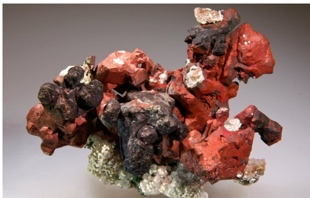
UM Copper Specimen from the Phoenix Mine, Keweenaw County MI. The red color comes from a thin coating of the mineral cuprite. Photo: Debra Wilson
