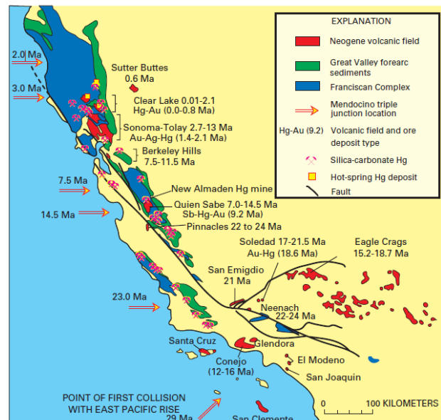
Mercury deposits in California mercury mineral belt. Fig. 12 from Rytuba, “Environmental Impact of Mercury Mines in the Coast Ranges, California”. http://pubs.usgs.gov/circ/2003/c1248/
